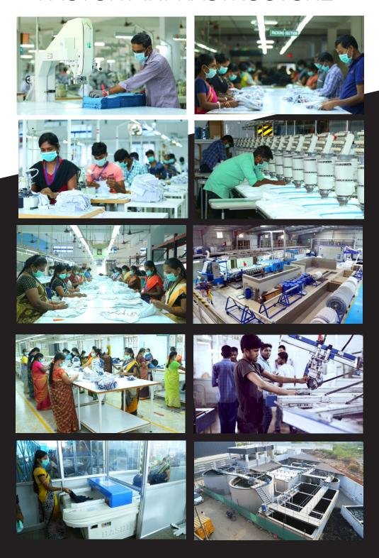
Cutting - Stitching - Trimming - Checking - Needle Detector -Finishing Embroidery - Rotary printing - Placement printing - RO plant
